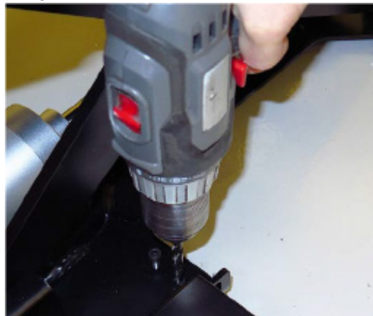
Figure 9: Use a 3/8 metal bit to drill bracket holes
