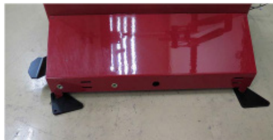
Figure 1: Place retainer plates under feet
