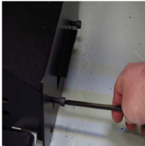
Figure 6: Secure guard to balancer
