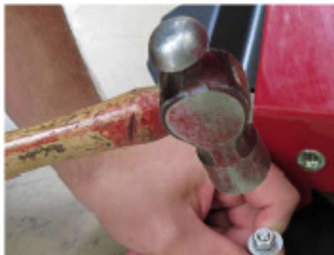
Figure 3: Hammer in stud
